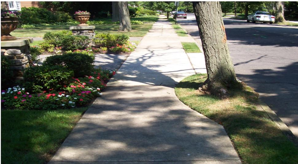
Minimum sidewalk width is 30 inches. The left edge of sidewalk can also be curved to maintain minimum width distance.
